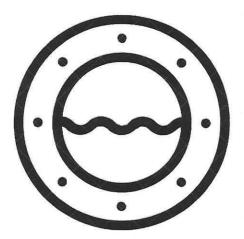
A **Porthole** in the ship is sometimes called a bull's-eye window, The function of a porthole, when open, is to permit light and fresh air to enter the dark and often damp belowdeck quarters of the vessel. It also affords below-deck occupants a limited view of the outside world when closed
