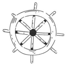
A **Shipboard Wheel** is a device used aboard a Ship to steer the vessel and control its course. Together with the rest of the steering mechanism, a large number of vessels appeared using the ship's wheel design near the beginning of the 18th century.
